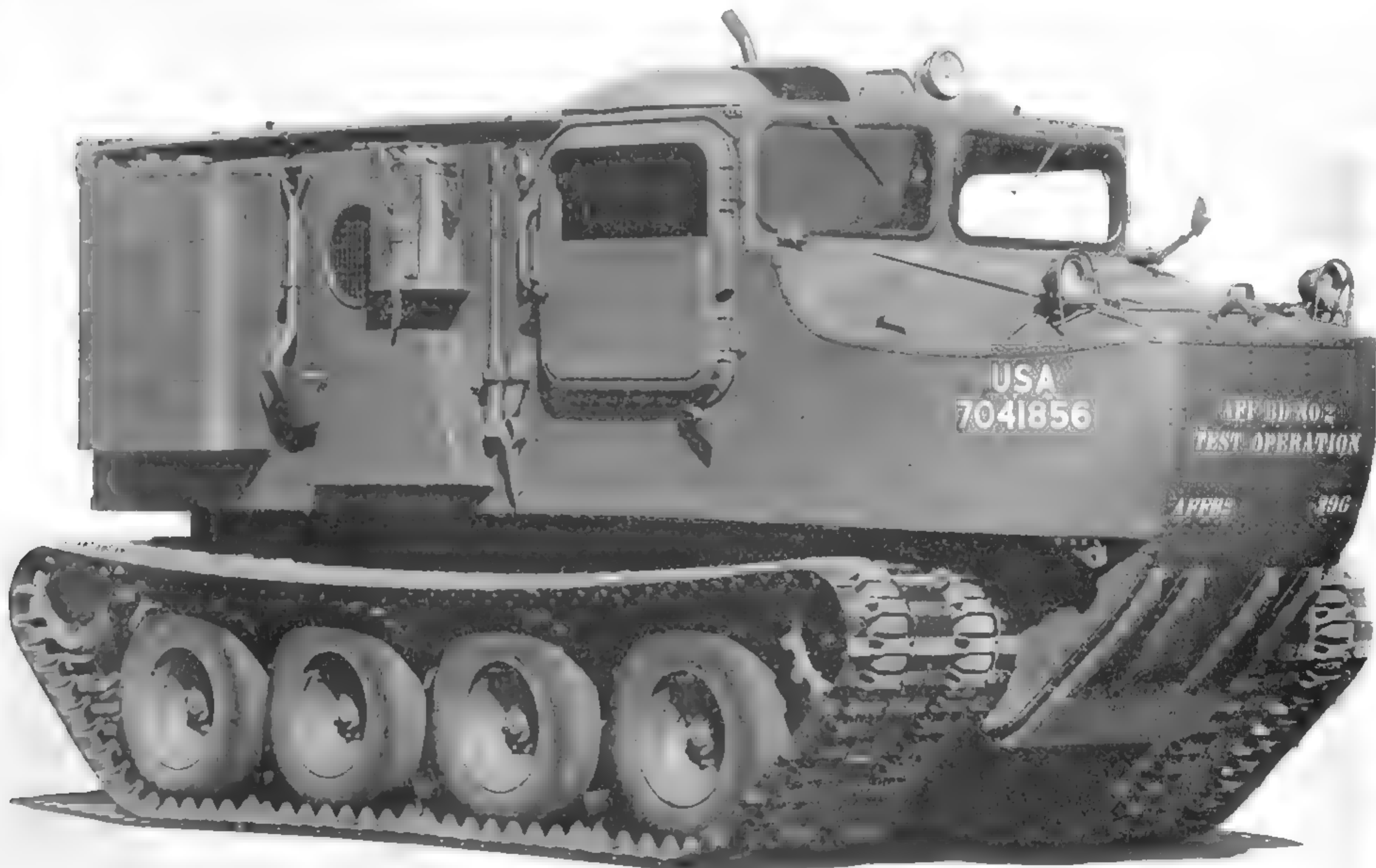
The M76 Otter was not only an unusually shaped vehicle, it had some unusual features as well. The road wheels were fully pneumatic tires, much like those on passenger cars, and the fuel tanks were mounted externally on the sides of the hull. One can be seen here as the bulging protrusion at the rear of the body. Also visible are the axe and mattock pioneer tools. (U.S. Army photo)
